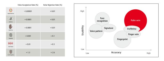
Compared to finger vein authentication, palm vein technology has 10 times the data points for superior security. External factors such as abrasians, hair, skin conditions, and water or lotions have little impact on the technology's ability to recognize an individual's identity.
