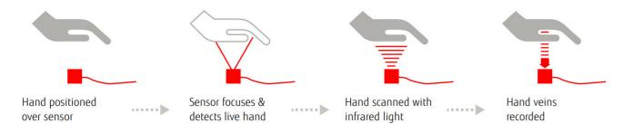
Palm vein authentication technology is the only internal biometric modality, making it virtually impossible to forge or spoof. With presentation attach detection and superior encryption, palm vein vascular recognition technology is the most secure form of biometric authentication. PalmSecure has significantly low false acceptance rates of 0.00001% and false read rates of 0.01%.
